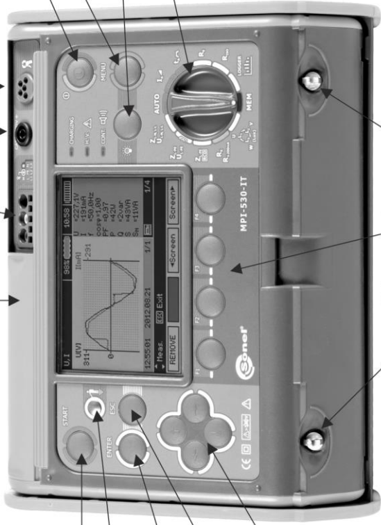
Start the measurement procedure Touch electrode Confirming the selection ESC - return to previous function, exit the function Shift/selection: right / left, up / down
